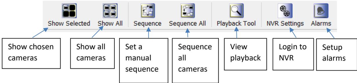
6. To login to NVR, select the NVR on left, and click "NVR Settings"
